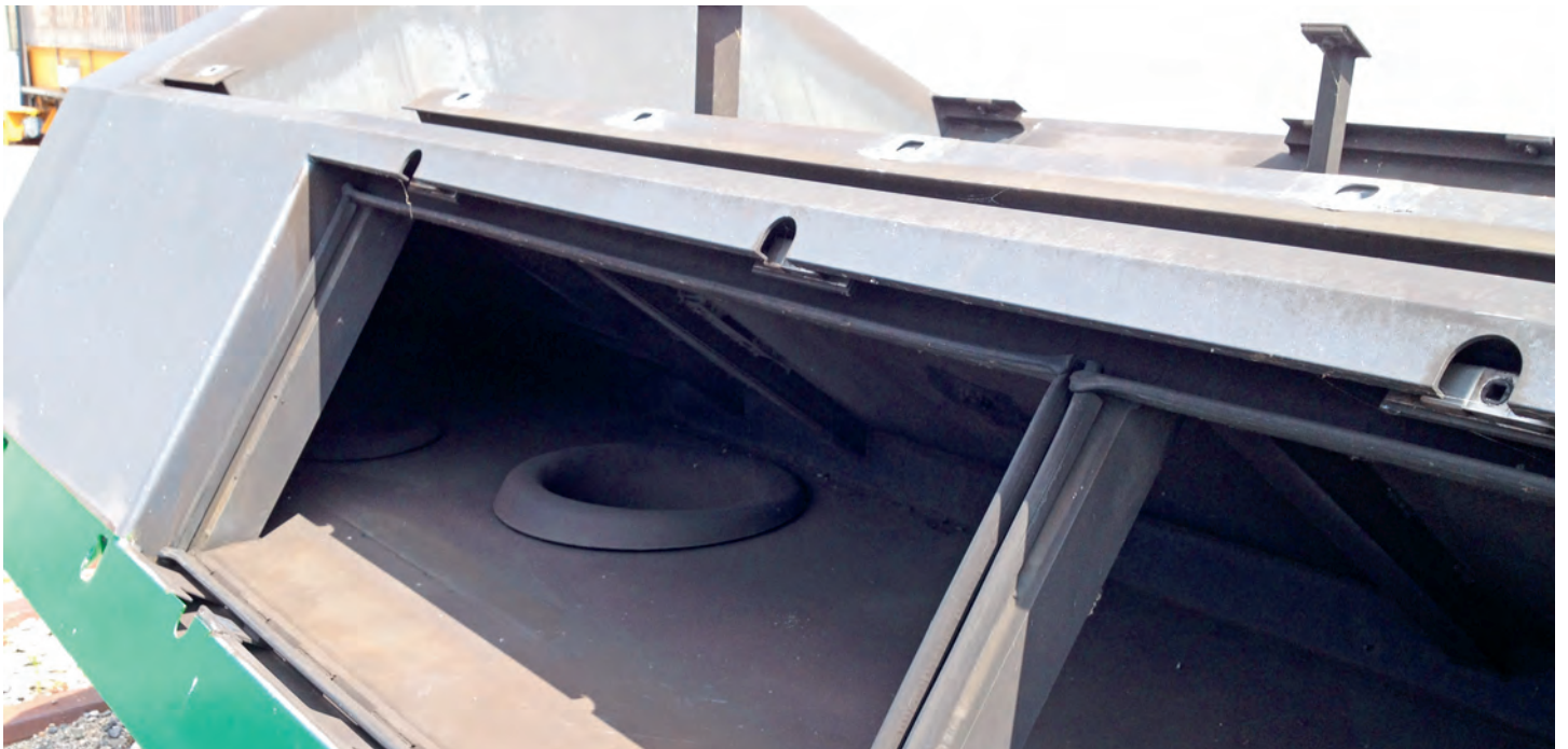
For maintenance the roof of the locomotive is removed. The original sealing frame for the filter grilles is clearly visible. It was cut to the correct length and glued to the corners.
