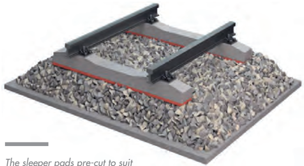
The sleeper pads pre-cut to suit the horizontal section of the sleeper.
